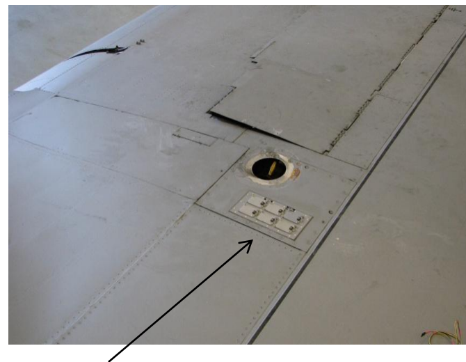
Panel with 6 sensors on C130; Upper Fuselage
