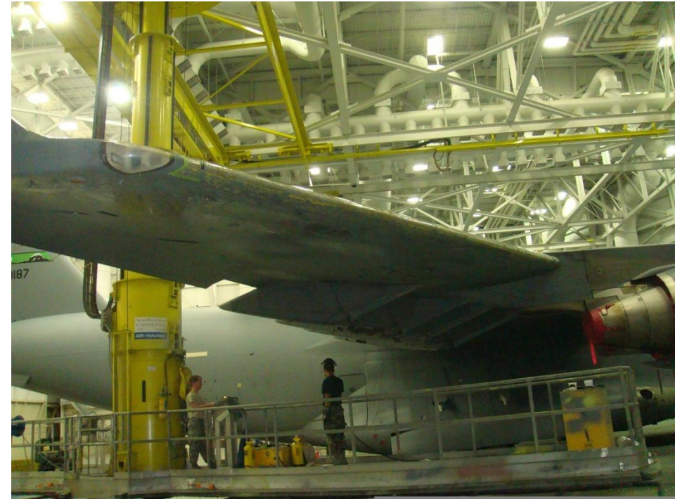
Test slats after alodine process
