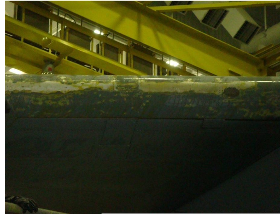
Test slats after alodine process
